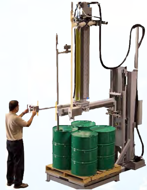
Twin-Lance Filler (Photo 1024) This twin lance drum and tote filler has a stainless lance for non-corrosives and a Kynar lance for acids. Extended lances allow bottom filling for tall containers, 5 to 550 gallon size from 20" to 80" tall. The see-through windshield is optional
